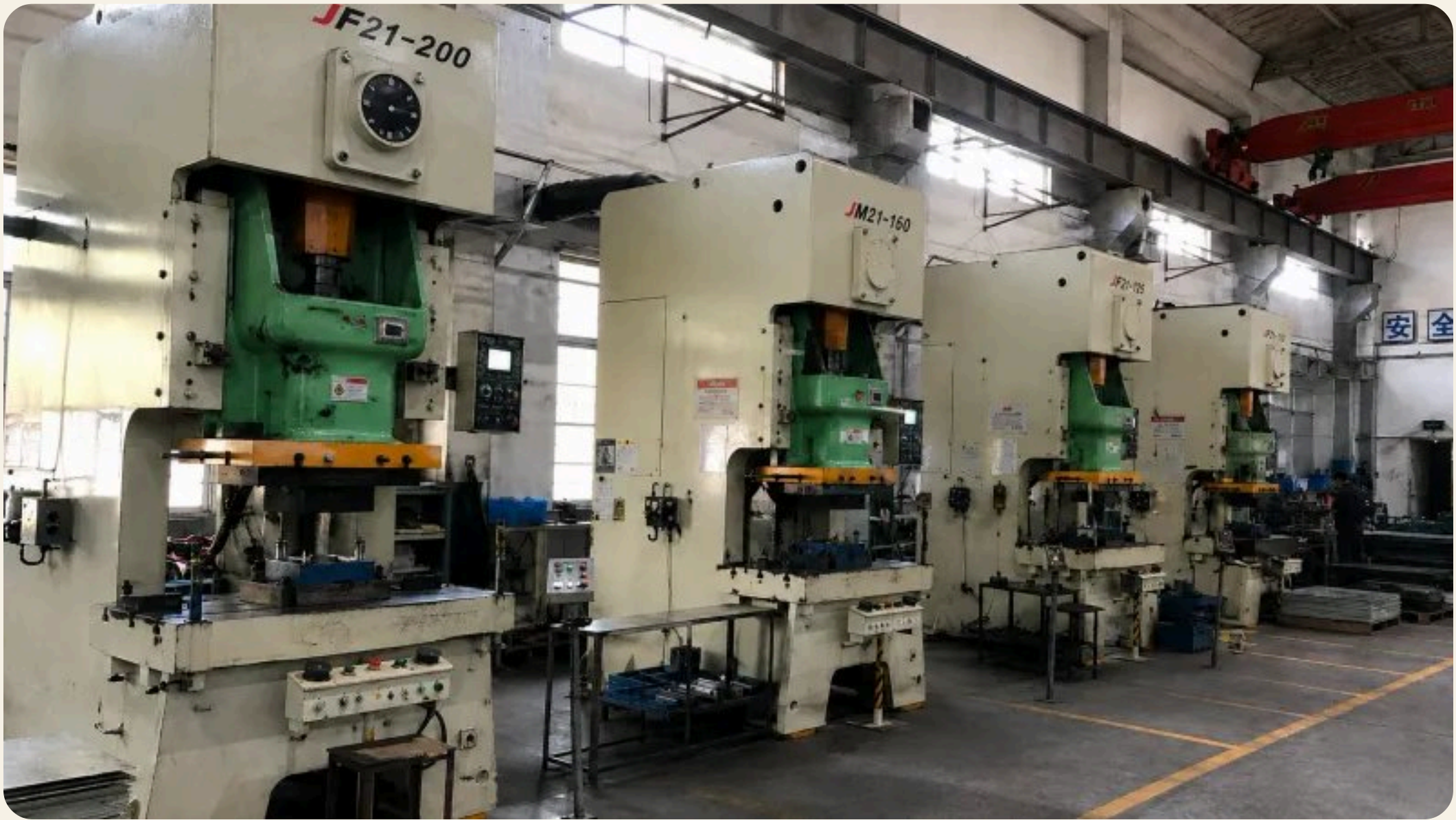
Mechanical press stamping line — 25T to 300T, up to 200 strokes per minute
