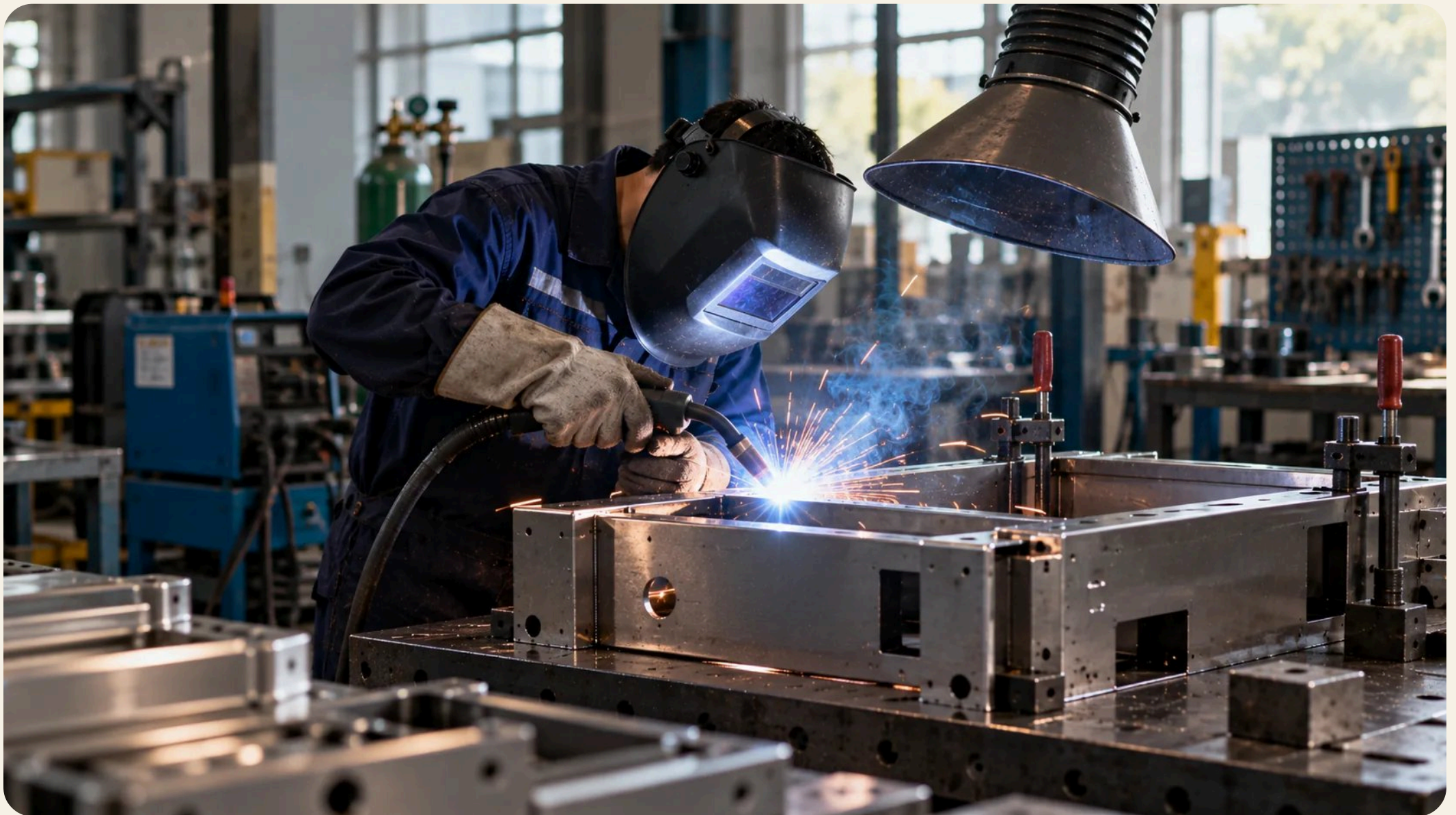
MIG welding a steel frame — continuous seam, IP65-capable
